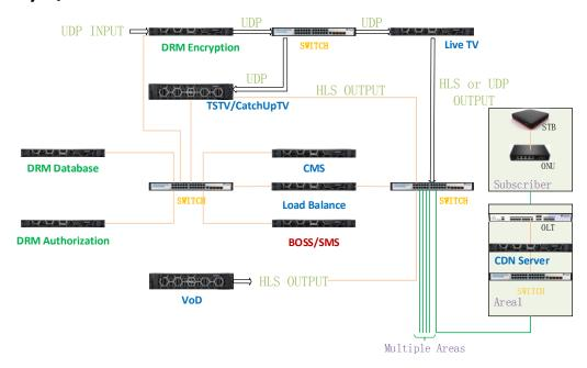
Gospell provides a Total IPTV Solution with a complete package tailored for operators without prior IPTV experience. This comprehensive solution includes a user-friendly Content Management System, robust DRM system, live streaming, video on demand, time-shift capabilities, catch-up TV, user management, CDN, Android set-top boxes, IPTV player, and a customizable launcher.
